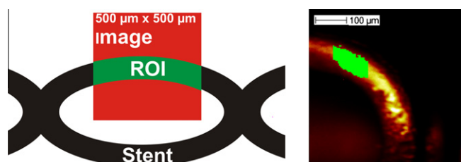
Fig. 6. Selection of analysis area and region of interest (ROI) in the performed depth profile measurement. Scheme of analysis area of TOF-SIMS measurement. The 500 \mu\text{m} times 500 \mu\text{m} imaging and sputtering area (red) in the left image was sketched in correlation to the stent. The analysis area (green) called region of interest (ROI) is shown in the schematics and in the two dimensional total ion image on the right side. The right image illustrates the ROI of the SIMS depth profile that was used for the preparation of the depth profile of Fig. 7. (For interpretation of the references to color in this figure legend, the reader is referred to the web version of this article.)
